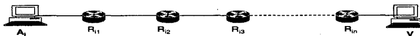
Figure 4.1 An instance of the attack traceback problem. The list of routers R_{i1}, R_{i2}, \dots, R_{in} represents the attack path followed by packets sent from A_i to V .
